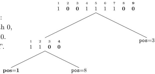
**Fig. 3.** Computing  $\pi^{-1}()$  on the runs-compressed data structure, using the example permutation of Fig. 2. We mark in bold the bits counted in the rank operations.
